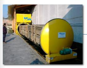
Vacuum and pressure phases are reached quickly, using powerful pumps to save time on cycle transitions.
