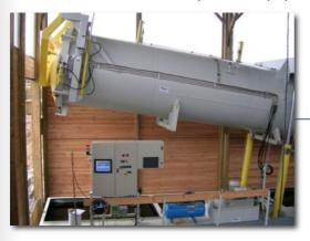
Touch panel is used for selection of user program and cycle start, along with cycle watch and maintenance functions. Cycle data recording using a networked desktop PC is available as an option.
