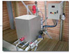
Tilting of vessel during final vacuum reduces draining time, increases the quantity of chemical return to the service tank, and keeps the draining area cleaner.
