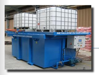
STAND ALONE SYSTEM FOR PREPARATION, MIXING, AND TRANSFER
