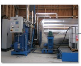
Cycle parameters can easily and accurately be adjusted. Water injection system allows treatment of a variety of wood species. A large fan ensures perfect heat distribution in the chamber.
